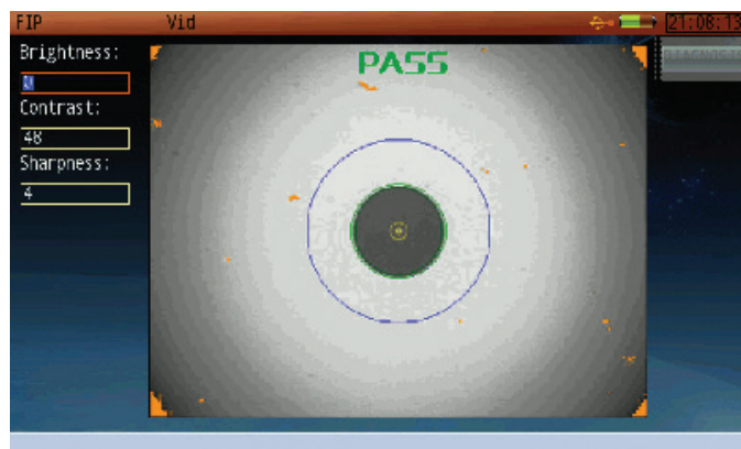
Figure 35: Inspect the face of the fiber optic connectors with the Fiberscope. Pass/Fail software interprets results.
