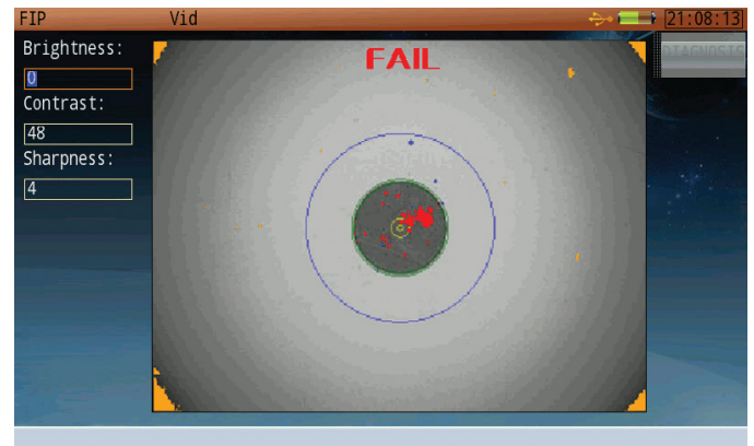
Figure 36: Fiberscope test with dirty connector.
