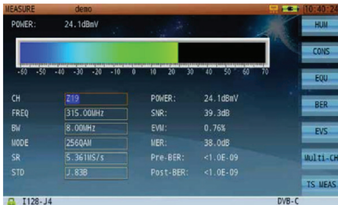
Figure 8: DVB-C channel measurements to characterize digital carrier metrics such as channel power, MER, Pre/Post BER.
