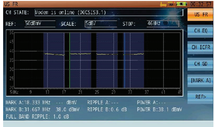
Figure 23: Use your own CMTS as your US sweep receiver, and get 256KHz of sweep resolution.
