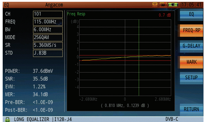
Figure 15: Frequency Response is derived from the adaptive EQ power coefficient. The in-band frequency response should not exceed ± 1.5 dB peak to valley.
