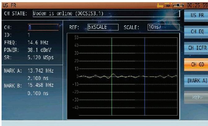
Figure 24: Get unprecedented Upstream Group delay from the integrated DS2831 US Cable Modem
